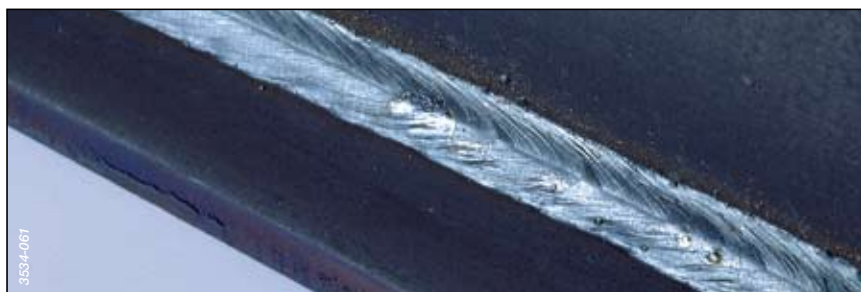
Lap joint welding in Speed Short Arc™ mode on 2 mm at 1.2 m/min.
